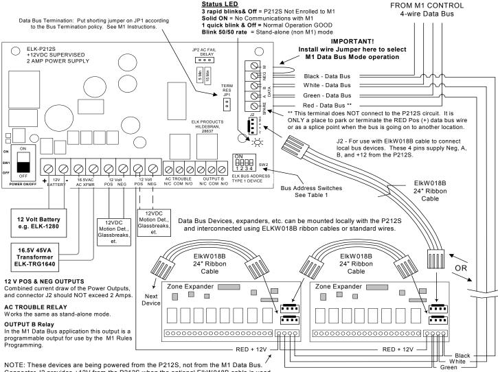
Connector J2 provides +12V from the P212S when the optional ElkW018B cable is used.
