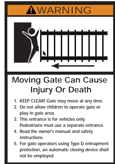
warning label (1) installed on operator housing
