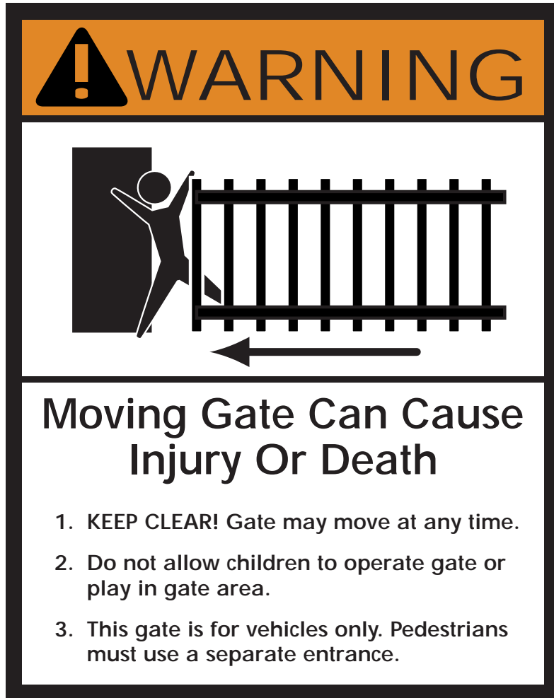
warning signs (2) to be installed on each side of the gate (3–5 feet above the bottom of the gate)
