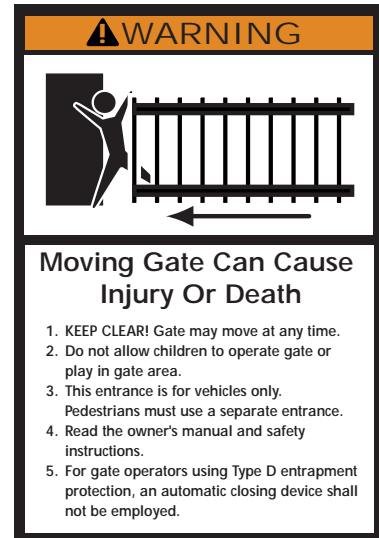
warning label (1) installed on operator housing
