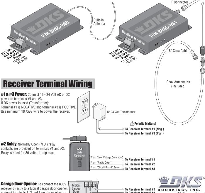
connect terminals 1, 2 and 3 on the receiver to Opener terminals 1, 2 and 3 on the garage door opener.
